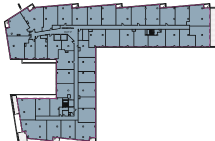
5. LEVEL 3 ELEVATION: 265'-0" GFA: 35,637 SF 1" = 50'-0"
